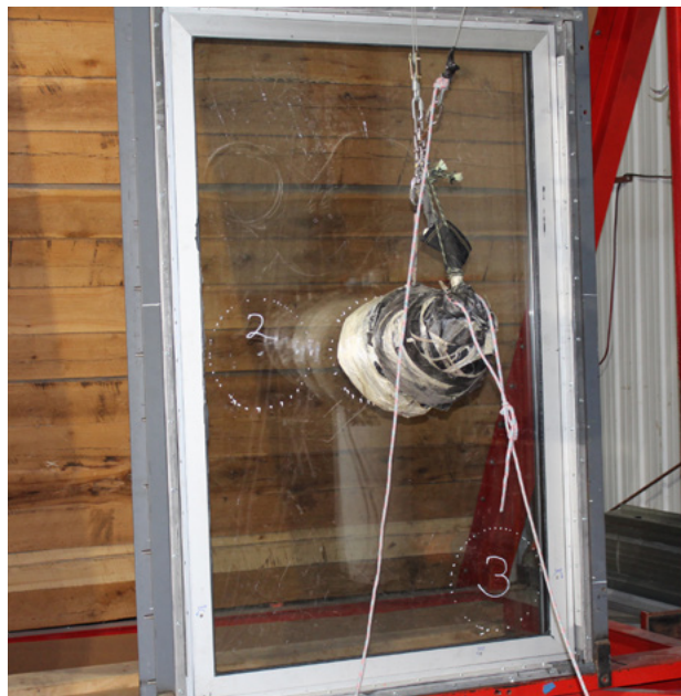
AAMA 501.8 Human Impact - a 300 lb bag is swung from 6'8" into the window to generate a 2,000 ft-lb impact
